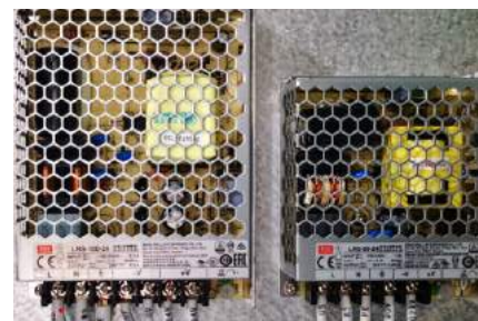
Double switching power supply
