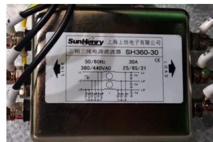
Three-phase three-wire power filter
